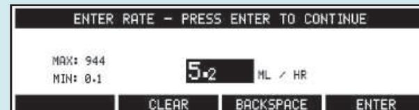
2. Use **CLEAR** or **BACKSPACE** to change the value. The **MAX** and **MIN** values show the programming limits. When the rate is correctly displayed, press **ENTER**. The limits are calculated by the pump.
